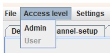
After selecting Admin and by entering the password. The default password to switch on the user level is "#01000".
