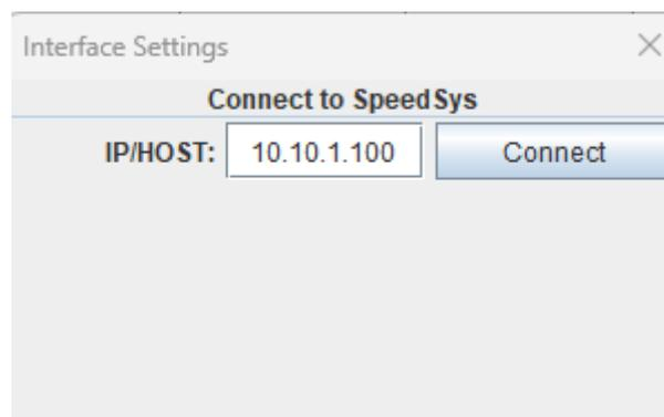
After clicking the 'Connect' button a connection is established, and the software is displaying the text 'Connected!' to indicate a successful connection has been made as shown in the figure below. Also, the buttons 'Read Configuration' and 'Write to Device' will become active.
