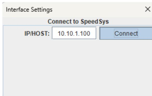
In the menu interface settings, the IP address of the connected SpeedSys Tx0 must be entered. After selecting "Connect", the unit will connect to the SpeedSys Tx0.
